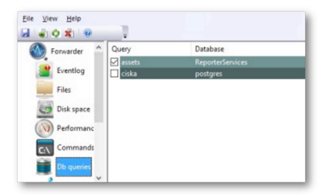
The Forwarder is able to run queries against any ODBC compliant database at defined intervals, and to stream the results of the query to the Arbitrator server.
