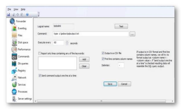
Special features have been added to handle the output from commands that produce CSV file types. It is strongly recommended that you select **Send command output one line at a time** for CSV formatted files
