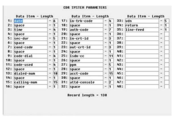
5. Change field 3 to start-time (length 6) and field 5 to end-time (length 6). Leave the rest of the fields as they were.
