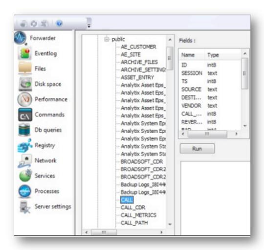
You can extend tables and views to see the database architecture. The tree structure will depend on the database layout and schemas (when applicable). Clicking on a table or view displays all the fields and their types:
